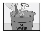
Mix 20kg TAL Goldstar HB tile adhesive with 5L of cool water. Using a mechanical mixer, mix to a creamy lump-free paste, while adding powder.
