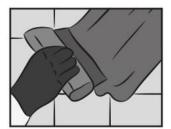
Grout after 14 - 16 hours with TAL Grout (as per instructions). Adhesive set should be achieved after 18 hours (in summer/warm ambient conditions). Allow for longer setting times when using larger format tiles or in cold ambient conditions.
