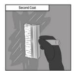
Apply the second coat of TAL SUREPROOF SHOWER in a cross direction to the first coat to ensure complete coverage, with no air entrapment or pinholes.
