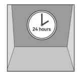
Allow the TAL SUREPROOF SHOWER system to dry completely (24-36 hours, depending on ambient and site conditions) before being subjected to light foot traffic or the application of tiles.
