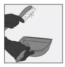
Ensure the surface is integrally sound, clean and free from any contamination such as dust, dirt, waxes, bituminous compounds and organic or fungal growth
