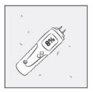
Ensure the moisture content of the shower walls and floor is less than 8%.
